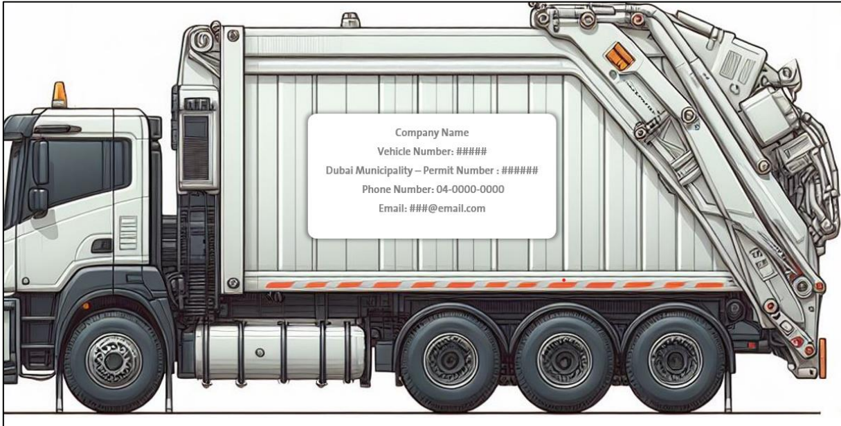
Figure 2 The right way to placard waste collection vehicles.
