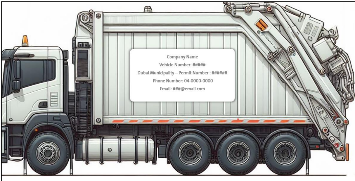
Figure 2 The right way to placard waste collection vehicles
