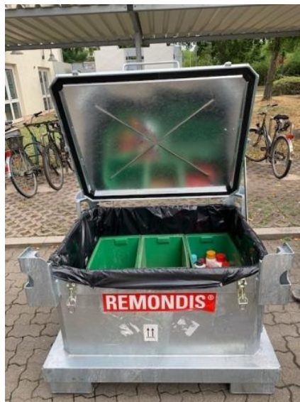
Figure 2 Sealed transport container with plastic bag as an additional collecting vessel for accidents
