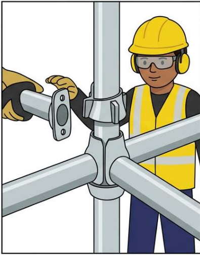
1- Locate the blade end of ledgers and transoms into cup.
