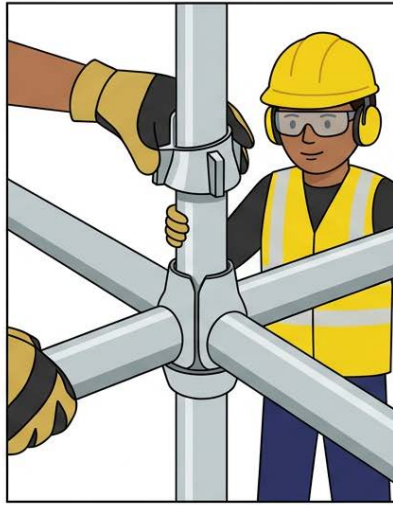
2- Lower the upper cup down the standard and rotate.
